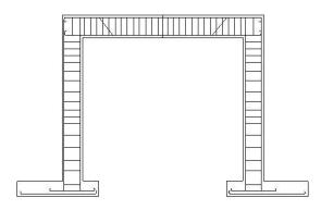
A : Portal frame with hinge baseB : Portal frame with fixed baseC : R.C.C framed structure
